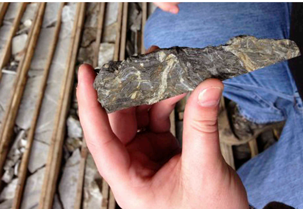
Drill core – Black Carbonaceous shale showing folding, at Clay Lake Gold Target
